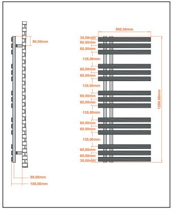
Dimensions (measurements in mm)
