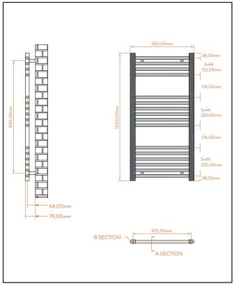
Dimensions (measurements in mm)
