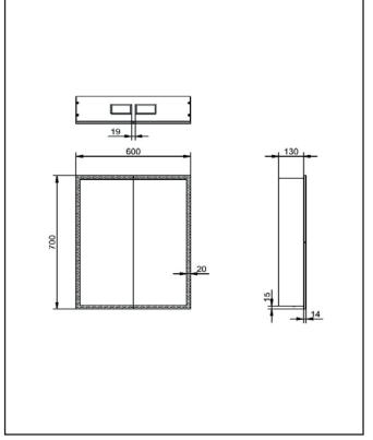
Dimensions (measurements in mm)
