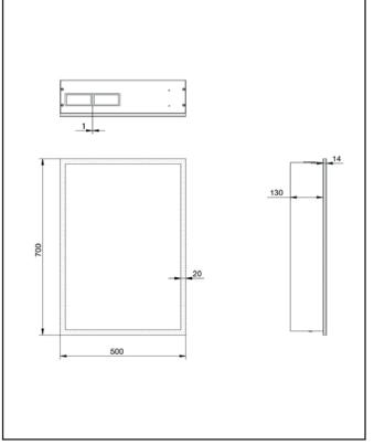
Dimensions (measurements in mm)
