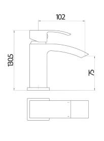
Dimensions (measurements in mm)
