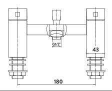
Dimensions (measurements in mm)
