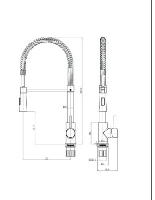
Dimensions (measurements in mm)
