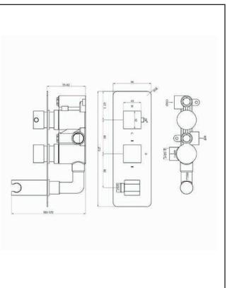
Dimensions (measurements in mm)
