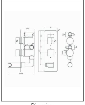
Dimensions (measurements in mm)
