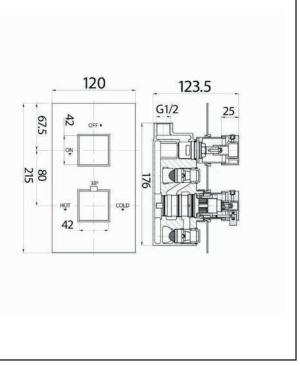
Dimensions (measurements in mm)
