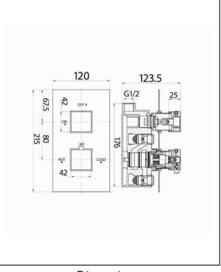
Dimensions (measurements in mm)
