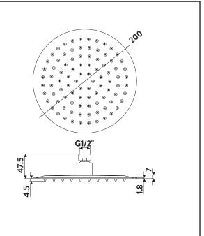
Dimensions (measurements in mm)
