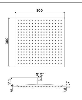
Dimensions (measurements in mm)
