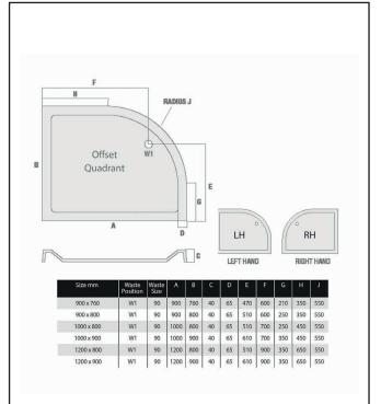
Dimensions (measurements in mm)
