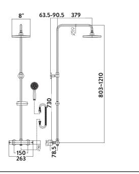
Dimensions (measurements in mm)
