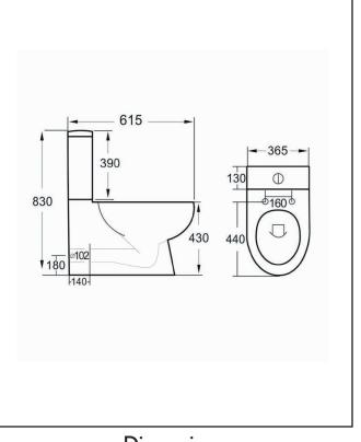
Dimensions (measurements in mm)
