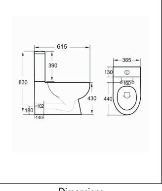
Dimensions (measurements in mm)
