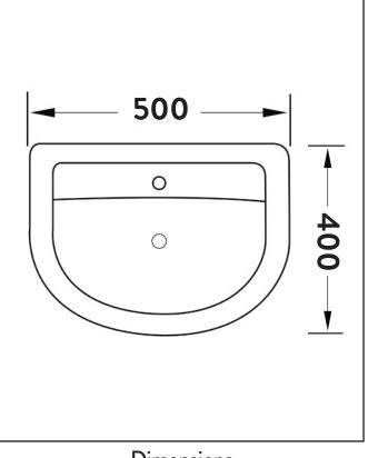
Dimensions (measurements in mm)
