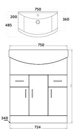
Dimensions (measurements in mm)
