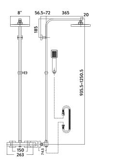
Dimensions (measurements in mm)
