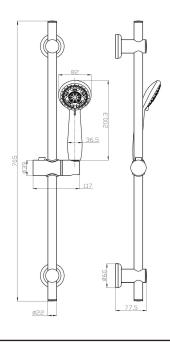
Dimensions (measurements in mm)
