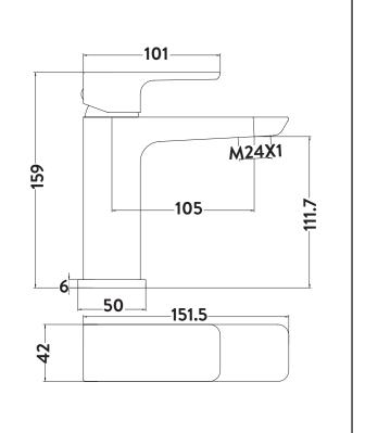
Dimensions (measurements in mm)
