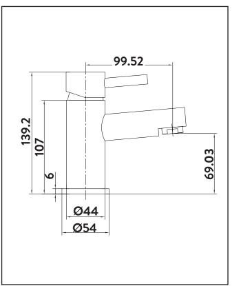
Dimensions (measurements in mm)
