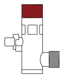
3. Use spanner to install hose onto shut off valve.
