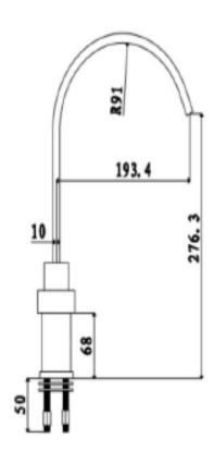
Dimensions: All measurements are in millimeters and are subject to normal manufacturing variations.
