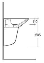
Dimensions: All dimensions in mm tollerance +5% for below 200mm and +3% for above 200mm.
