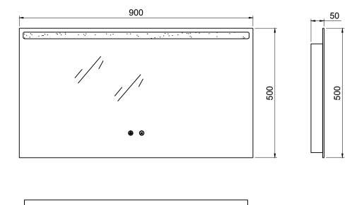
Dimensions: All measurements are in millimeters and are subject to normal manufacturing variations.
