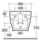
Dimensions: All dimensions in mm tolerance  $\pm 5\%$  for below 200mm and  $\pm 3\%$  for above 200mm. Note: Due to a continuing development programme to improve design and performance, the manufacturer reserves all rights to vary specifications without prior information.
