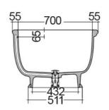
Dimensions: All dimensions in mm tolerance ±5% for below 200mm and ±3% for above 200mm.
