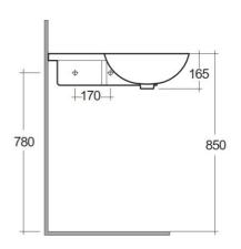
Dimensions: All dimensions in mm tolerance  $\pm 5\%$  for below 200mm and  $\pm 3\%$  for above 200mm. Note: Due to a continuing development programme to improve design and performance, the manufacturer reserves all rights to vary specifications without prior information.
