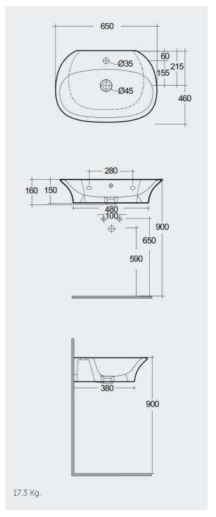
Dimensions: All dimensions in mm tolerance  $\pm 5\%$  for below 200mm and  $\pm 3\%$  for above 200mm. Note: Due to a continuing development programme to improve design and performance, the manufacturer reserves all rights to vary specifications without prior information.
