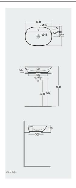
Dimensions: All dimensions in mm tolerance ±5% for below 200mm and ±3% for above 200mm.
