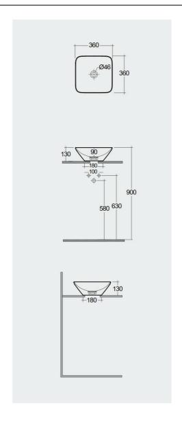
Dimensions: All dimensions in mm tolerance ±5% for below 200mm and ±3% for above 200mm.
