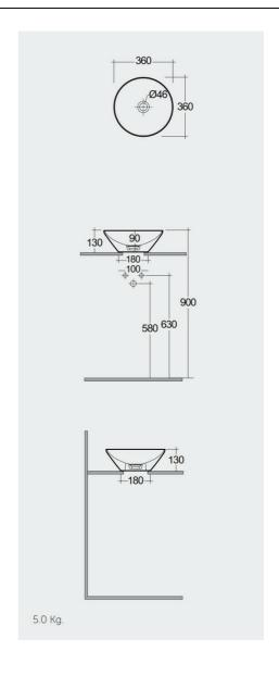
Dimensions: All dimensions in mm. Tolerance of vitreous china & fireclay items:  $\pm$  5% for below 200mm and  $\pm$  3% for above 200mm; for all other items tolerance  $\pm$  1%. Note: Due to a continuing development program to improve design and performance, the manufacturer reserves all rights to vary specifications without prior information. Please note accessories are for photographic use only.
