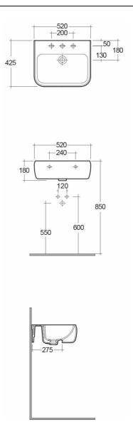
Dimensions: All dimensions in mm. Tolerance of vitreous china & fireclay items: ± 5% for below 200mm and ± 3% for above 200mm; for all other items tolerance ± 1%. Note: Due to a continuing development program to improve design and performance, the manufacturer reserves all rights to vary specifications without prior information. Please note accessories are for photographic use only.
