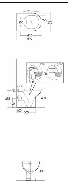
Dimensions: All dimensions in mm. Tolerance of vitreous china & fireclay items:  $\pm$  5% for below 200mm and  $\pm$  3% for above 200mm; for all other items tolerance ± 1%. Note: Due to a continuing development program to improve design and performance, the manufacturer reserves all rights to vary specifications without prior information. Please note accessories are for photographic use only.
