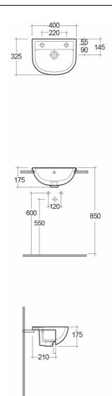
Dimensions: All dimensions in mm. Tolerance of vitreous china & fireclay items: ± 5% for below 200mm and ± 3% for above 200mm; for all other items tolerance ± 1%. Note: Due to a continuing development program to improve design and performance, the manufacturer reserves all rights to vary specifications without prior information. Please note accessories are for photographic use only.
