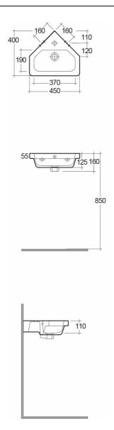
Dimensions: All dimensions in mm. Tolerance of vitreous china & fireclay items:  $\pm$  5% for below 200mm and  $\pm$  3% for above 200mm; for all other items tolerance  $\pm$  1%. Note: Due to a continuing development program to improve design and performance, the manufacturer reserves all rights to vary specifications without prior information. Please note accessories are for photographic use only.
