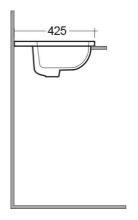
Dimensions: All dimensions in mm tolerance  $\pm 5\%$  for below 200mm and  $\pm 3\%$  for above 200mm. Note: Due to a continuing development programme to improve design and performance, the manufacturer reserves all rights to vary specifications without prior information.
