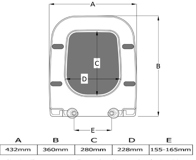
Dimensions: All measurements are in millimeters and are subject to normal manufacturing variations.
