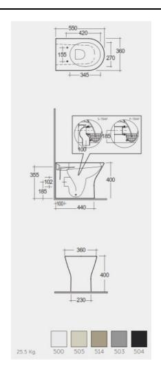
Dimensions: All dimensions in mm. Tolerance of vitreous china & fireclay items: ± 5% for below 200mm and ± 3% for above 200mm; for all other items tolerance ± 1%. Note: Due to a continuing development program to improve design and performance, the manufacturer reserves oll rights to vary specifications without prior information. Please note accessories are for photographic use only.
