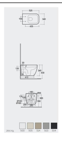
Dimensions: All dimensions in mm. Tolerance of vitreous china & fireclay items: ± 5% for below 200mm and ± 3% for above 200mm; for all other items tolerance ± 1%. Note: Due to a continuing development program to improve design and performance, the manufacturer reserves oll rights to vary specifications without prior information. Please note accessories are for photographic use only.
