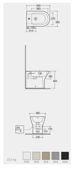
Dimensions: All dimensions in mm tolerance  $\pm 5\%$  for below 200mm and  $\pm 3\%$  for above 200mm. Note: Due to a continuing development programme to improve design and performance, the manufacturer reserves all rights to vary specifications without prior information.
