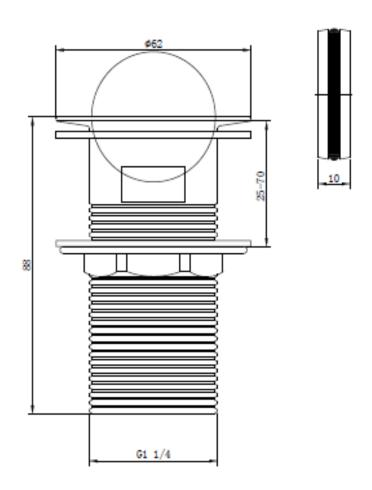
Dimensions: All measurements are in millimeters and are subject to normal manufacturing variations.
