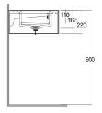
Dimensions: All dimensions in mm. Tolerance of vitreous china & fireclay items: ± 5% for below 200mm and ± 3% for above 200mm; for all other items tolerance ± 1%. Note: Due to a continuing development program to improve design and performance, the manufacturer reserves all rights to vary specifications without prior information. Please note accessories are for photographic use only.
