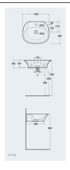
Dimensions: All dimensions in mm. Tolerance of vitreous china & fireclay items: ± 5% for below 200mm and ± 3% for above 200mm; for all other items tolerance ± 1%. Note: Due to a continuing development program to improve design and performance, the manufacturer reserves all rights to vary specifications without prior information. Please note accessories are for photographic use only.
