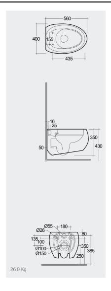
Dimensions: All dimensions in mm. Tolerance of vitreous china & fireclay items: ± 5% for below 200mm and ± 3% for above 200mm; for all other items tolerance ± 1%. Note: Due to a continuing development program to improve design and performance, the manufacturer reserves all rights to vary specifications without prior information. Please note accessories are for photographic use only.
