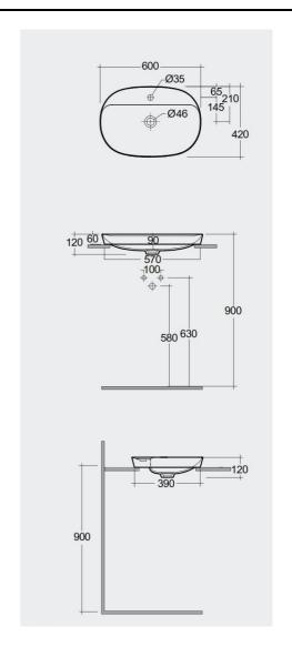
Dimensions: All dimensions in mm. Tolerance of vitreous china & fireclay items: ± 5% for below 200mm and ± 3% for above 200mm; for all other items tolerance ± 1%. Note: Due to a continuing development program to improve design and performance, the manufacturer reserves all rights to vary specifications without prior information. Please note accessories are for photographic use only.
