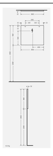
Dimensions: All dimensions in mm. Tolerance of vitreous china & fireclay items: ± 5% for below 200mm and ± 3% for above 200mm; for all other items tolerance ± 1%. Note: Due to a continuing development program to improve design and performance, the manufacturer reserves all rights to vary specifications without prior information. Please note accessories are for photographic use only.
