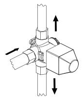
Fix the valve in the installation cube horizontally after spirit lever measuring.
