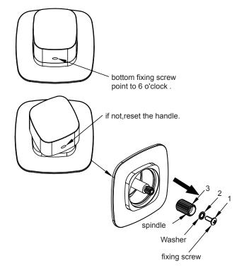
Make sure the bottom fixing screw always point to 6 o'clock when switch off. If not, disassemble the handle cap and parts #1 - #3 as arrow direction, rotate the spindle, until the handle could be set in correct direction.
