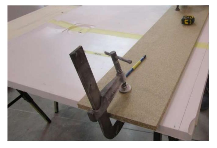
Fix the panel with clamps overlapping it with the offset line
