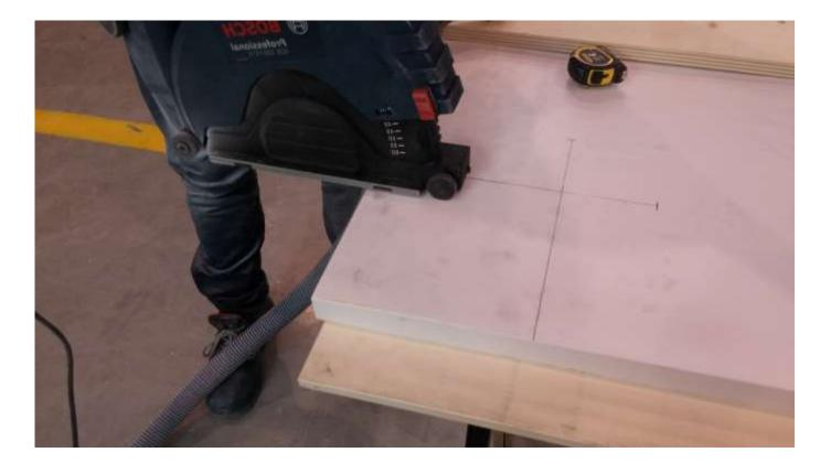
Proceed with cutting along the traced lines, referring to the cutting indicator on the tool. Be careful to stop with the blade <u>before</u> the intersection
