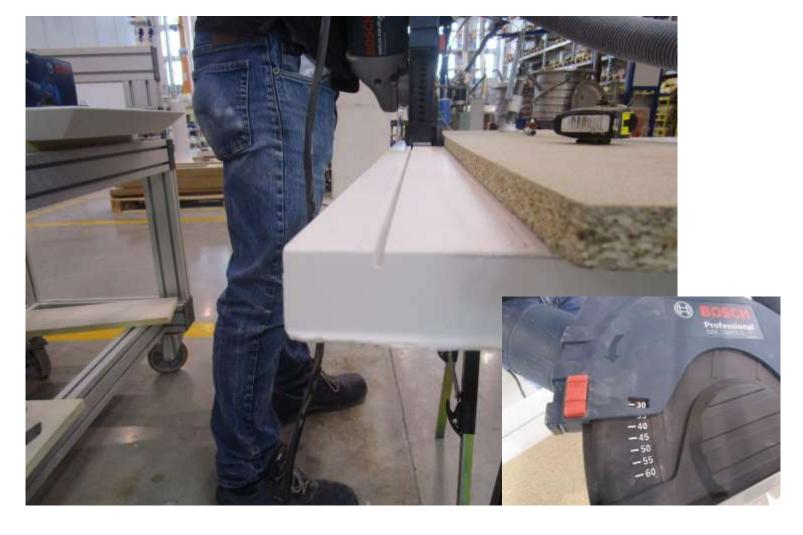
Make a first 10 mm cut on the upper surface and on the edges. Adjust tool settings properly.
