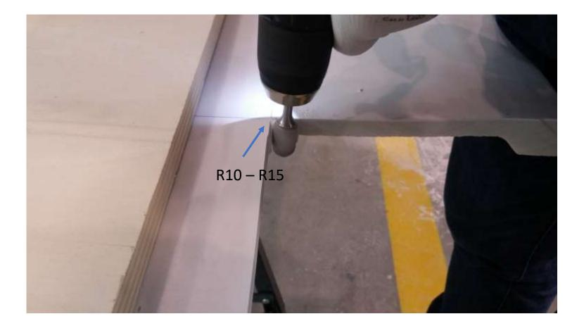
Remove irregularities using a cutter and make radius (minimum R10 – suggested R15)
