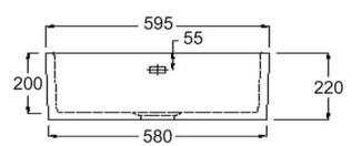
NB: Due to manufacturing processes this sink may have a +/- 5mm tolerance on the measurements provided
